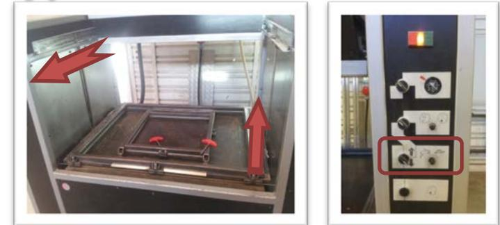
Fit the plastic plate on the frame. Pull back the top and then raise the frame.
