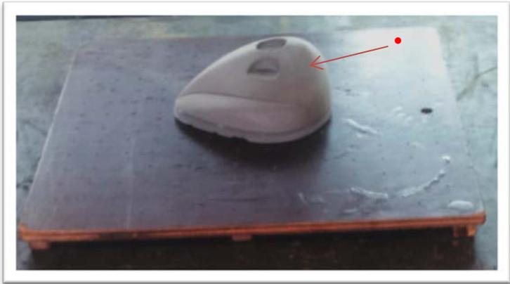
Place the model centered and ensure that there is adequate air holes positioned around the model.
